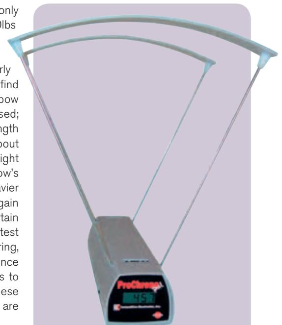
A chronograph can be used to measure how fast an arrow travels in fps
