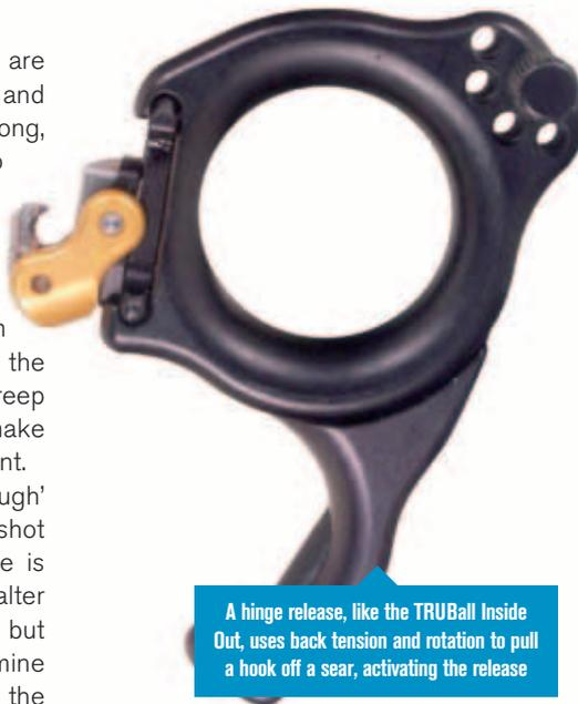
A hinge release, like the TRUBall Inside Out, uses back tension and rotation to pull a hook off a sear, activating the release
